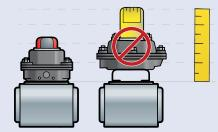
Low Profile Design The unique directmounting feature eliminates expensive mounting brackets while reducing the height of the switchbox and the overall footprint above the actuator.
